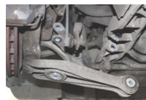
Drop the arm down to access the Ball joint
