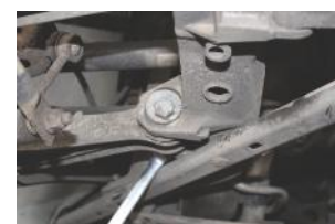
Remove the inner bush bolt
