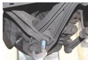
Remove the outer bush bolt removing control arm link to arm
